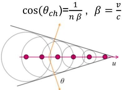
Schematic of Cherenkov radiation produced in cone-like shape from a particle. Taken from [4].
